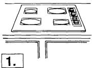
Insert the cooktop into the countertop cutout. Center the cooktop in the cutout. Check that the front of the cooktop is parallel to the front edge of the countertop. Check that all required clearances are met. If cooktop is not properly positioned, lift the entire cooktop out of opening to make adjustments.
